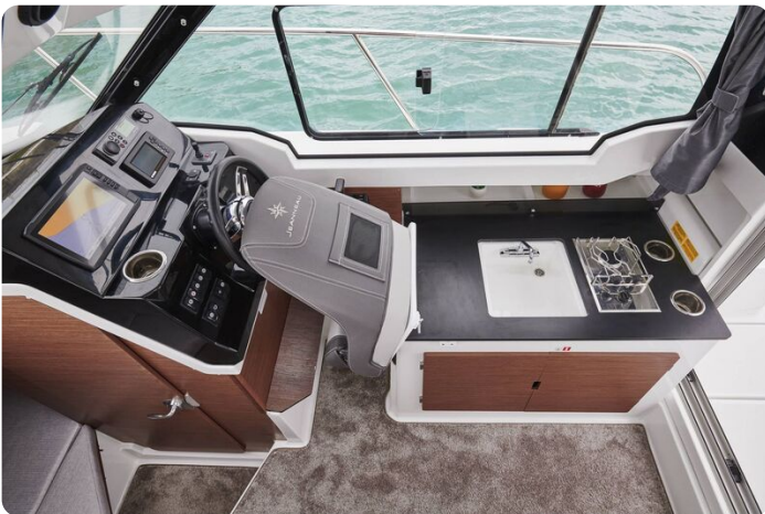
Jeanneau Merry Fisher 795 Series 2 - helm seat folds forward for easy access to galley
